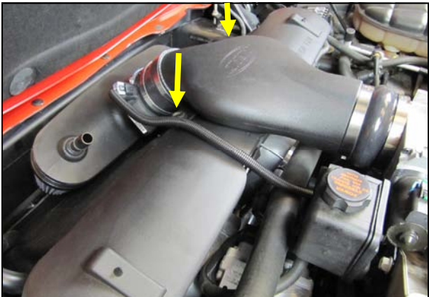
13. Slide the coupler all the way down onto the MAF and secure the Intake grommets onto the posts on the radiator shroud.
