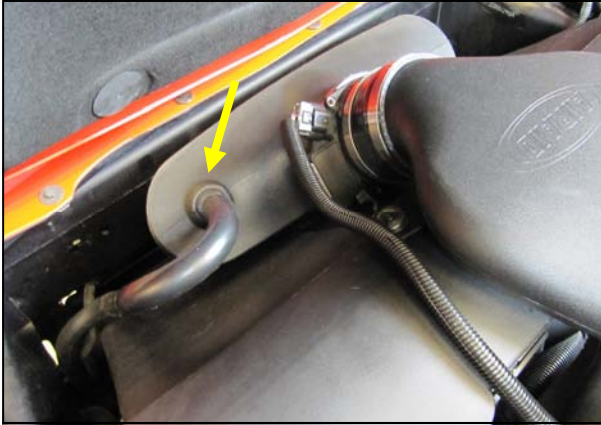
14. Connect the air pump breather line to the coupling on the Filter assembly.
