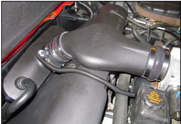
15. Check the alignment of all the intake components and adjust if necessary. Begin tightening the clamps from the front of the intake and move back towards the throttle body. Reconnect the battery.
