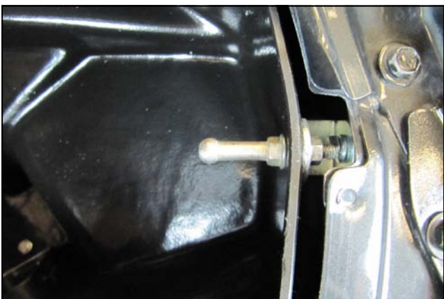
11. Reinstall the factory ground lug through the Cool Air Box and through the Side Bracket using one 1/4 " Flat Washer and the 6mm Flange Nut (#22).
