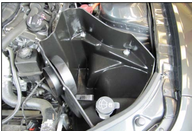
10. Install the Cool Air Box assembly into the vehicle. Slide the airbox grommets and sleeves over the factory studs and secure it using the nuts removed in step 3. Hint: Lifting the washer bottle cap makes for an easier installation.
