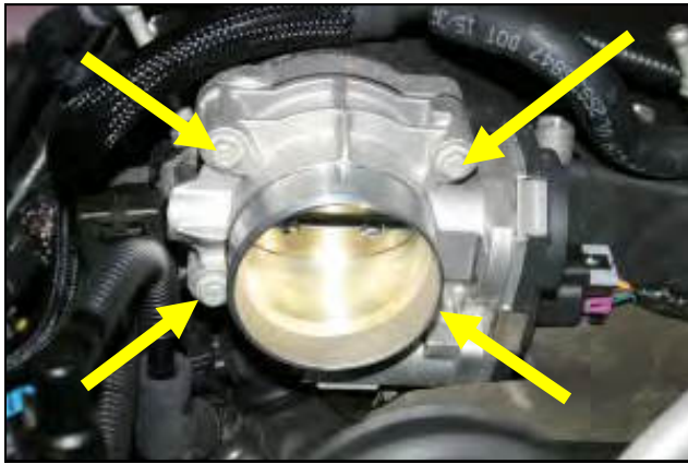
3. Remove the four bolts that secure the throttlebody to the intake manifold.
