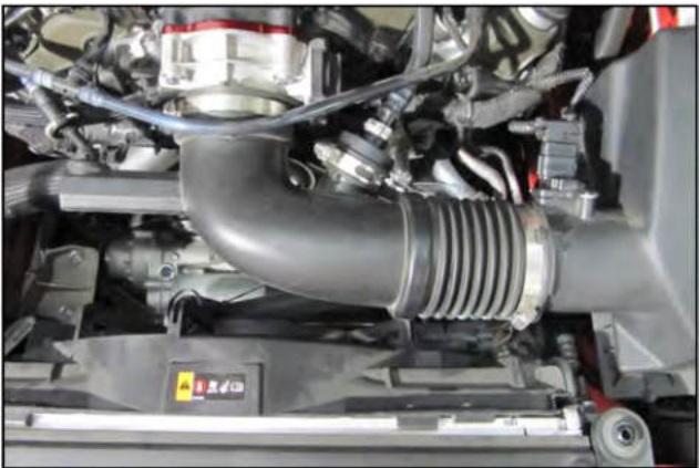
7. Reinstall the intake tube, tighten the two hose clamps, and reconnect the crankcase breather tubes. Reinstall the beauty cover, and oil cap in the reverse order in which they were removed.
