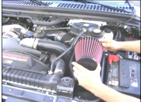
15. Install the Airaid Premium Filter (#1) onto the Airaid Intake Tube inside of the airbox, and tighten the hose clamp.
