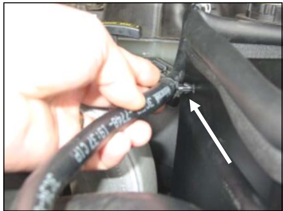
18. Spread the black hose mount (#8) over the radiator overflow hose and insert the tab through the hole in the side of the top panel.
