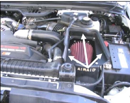
17. Install the weather strip (#5) around the edges of the top panel. ( Hint: Start at one corner of the panel and work to the other end. )
