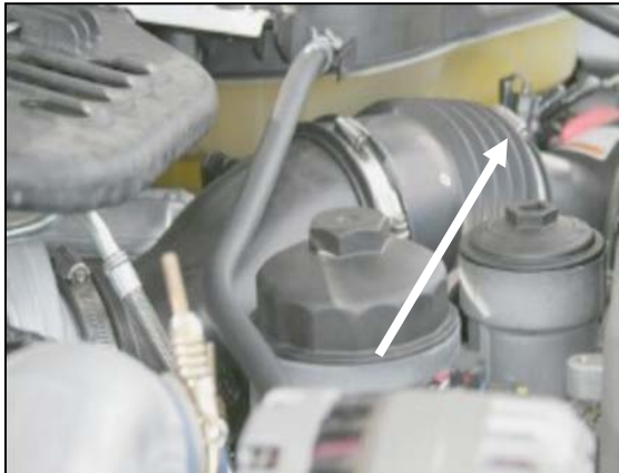
13. Tighten the hose clamp where the factory flexible turbo inlet tube slides over the Airaid Intake Tube.
