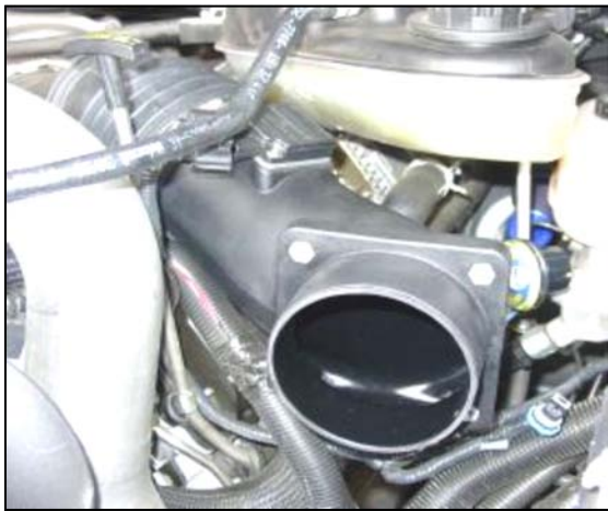
10. Slide the Airaid Intake Tube (#3) into the factory flexible turbo inlet hose. ( Note: Do not tighten the hose clamp until assembly is complete. ) Reconnect the sensor wiring harness (to the temperature sensor, or the MAF sensor, whichever is present on your vehicle.)
