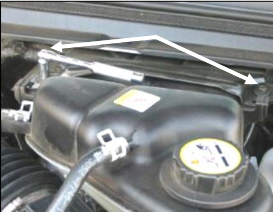
14. Factory tolerances may vary between the MAF sensor and the coolant reservoir. Therefore, it may be necessary to loosen the two 5/16" mounting bolts and adjust the reservoir for better clearance.
