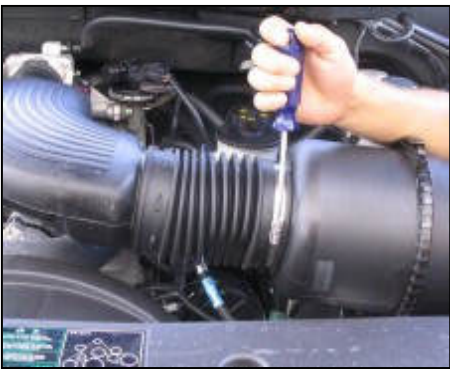
15. Loosen hose clamps connecting the factory intake tube to the air filter assembly and throttle body.
