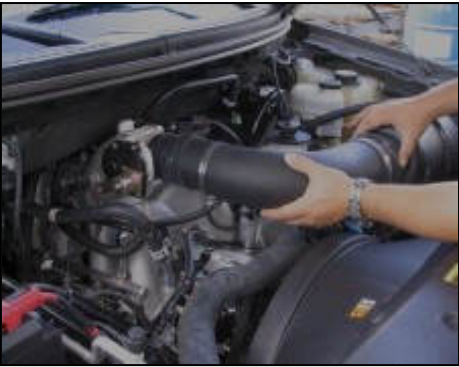
19. Install the Airaid Modular Intake Tube on engine.
