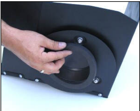
5. Install the supplied gasket on the Airaid filter adapter as shown.
