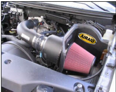
22. Double-check your work to be certain that all nuts, bolts, and clamps are securely fastened. Check for proper hood clearance before shutting hood.
