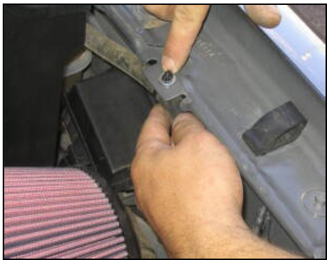
13. Mount the factory coolant hose to the inner fender using the supplied black plastic hose mount and washer as shown above.
