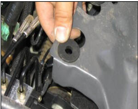
7. Install the supplied rubber grommets in place of the factory grommets previously removed.
