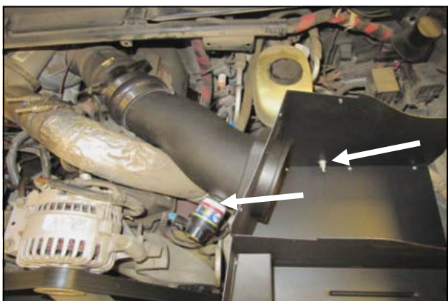
10. Insert the Airaid Intake Tube into the CAD assembly, then slide the Hump Hose onto the turbo inlet and tighten the Clamps. Reconnect the filter minder and the air temp sensor.
