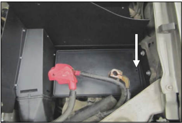
14. Place the Battery Mat (#7) into the CAD assembly with drain tube on the Drivers side.
