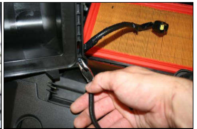
3. Using a pair of needle nose pliers, carefully compress the fins of the wiring harness anchor and pull it out of the air box lid.
