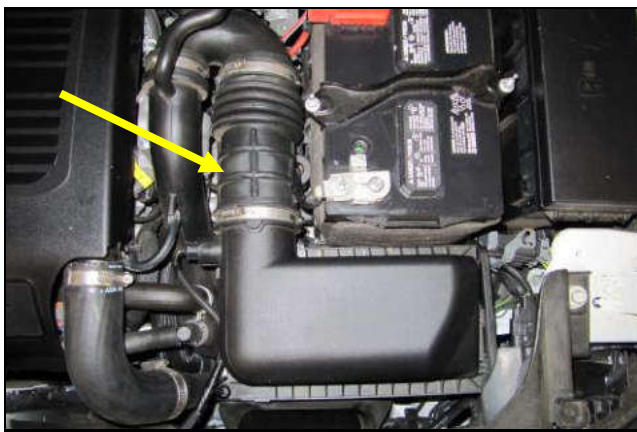
1. Disconnect the negative battery cable. Loosen the clamp on the air box side of the intake tube.
