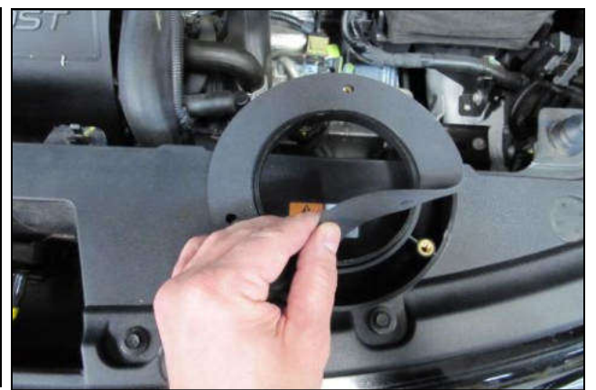
6. Prepare the Filter Adapter for installation by positioning the Adapter Gasket on the mounting side and lining up the holes.
