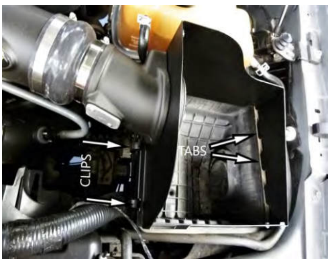
12. Install the Tube and Panel assembly onto the Airaid Intake Tube first, then insert the Panel tabs into the factory air box slots. Adjust the assembly until the OEM air box clips can positively engage the Panels and lock.
