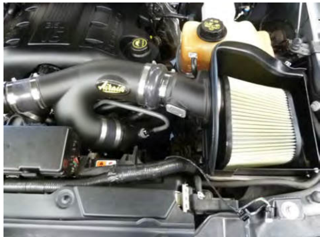
15. Double check your work. Make sure there is no foreign material in the intake path. Make sure all clamps, hoses, bolts, and screws are tight. Double check the hood clearance. Reconnect the negative battery cable.
