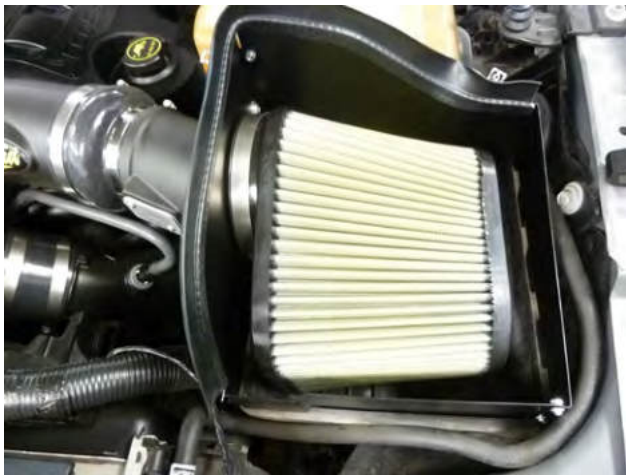
14. Install the Airaid Premium Filter onto the Sensor Tube and tighten the clamp.
