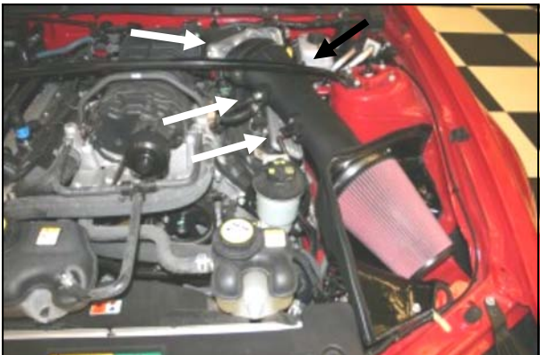
15. Adjust the Airaid Intake Tube for fit and then tighten the hose clamps on the throttlebody and the tube. Now reconnect the wiring harness to the MAF, the breather to the aluminum fitting, and the vacuum hose to the barbed fitting on the Airaid Intake Tube.
