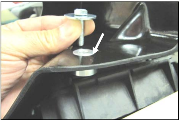
12. Slide the Aluminum Spacer (#12) underneath the CAD and into the hole as shown. Secure the CAD to the inner fender using the OEM bolt from step #1 and the supplied 1/4" Fender Washer (#10).
