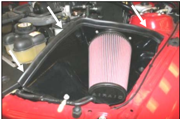
14. Install the Airaid Premium Filter (#1) onto the Airaid Intake Tube and tighten the hose clamp. Next install the supplied weather strip (#5) onto the top of the CAD as shown. For ease of installation, start next to the radiator and work your way towards the fender.
