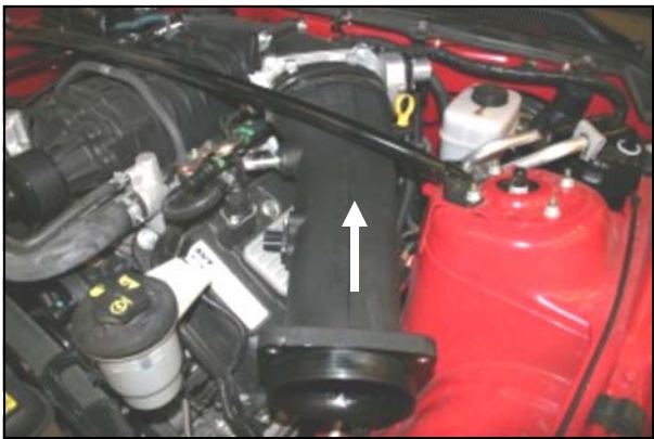
11. Install the Airaid Intake Tube into the oval hump hose. For ease of installation, don't tighten the clamps yet!
