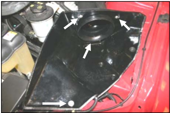
13. Install the Cool Air Dam into the vehicle aligning the grommet posts on the bottom of the CAD into the factory grommets in the fender well. Now install three 1/4" button head bolts (#6) and flat washers (#7) thru the CAD and into the Airaid Intake Tube. Next reinstall the second factory bolt from step #6 into its respective hole.
