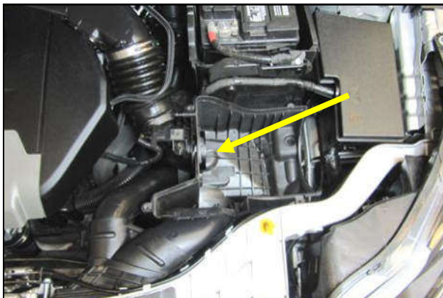
4. Notice how the OEM filter is installed in the air box . Remove the factory air filter and examine the mounting tube inside the air box.
