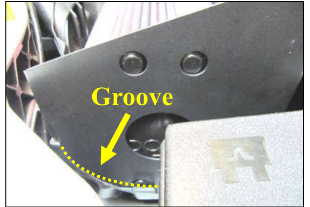
12. When properly installed, the panel will reside inside the groove in the air box and both sets of locating lugs will positively engage the holes in the Panel.
