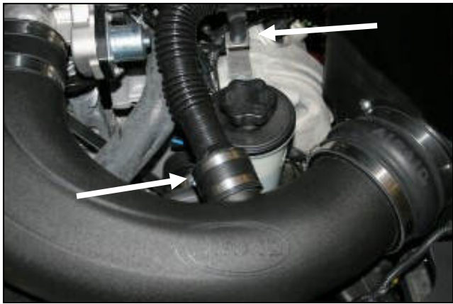
13. Install the air intake tube into the hump hose first, and then onto the throttlebody. Adjust for fit and then tighten all four hose clamps. Next, reinstall the factory resonator tube into the 1 3/4" coupler and tighten the hose clamp. Now "reseat" the resonator tube onto the bracket.
