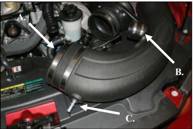
12.A.) Install the oval coupler onto the intake tube using two #72 hose clamps (#15). Leave the clamps loose for now. B.) Install the 1 3/4" coupler (#6) onto the intake tube using two #28 hose clamps (#16) as shown. Tighten only the clamp against the tube for now. C.) Install the provided grommet (#17) into the intake tube and then install the aluminum fitting (#20) into the grommet as shown.
