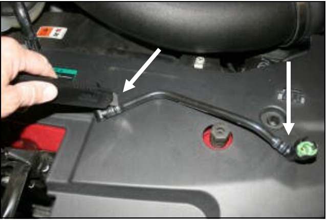
15. VERY CAREFULLY! Without cutting thru the connectors, cut the factory breather tube on each end just enough to remove the factory connectors.
