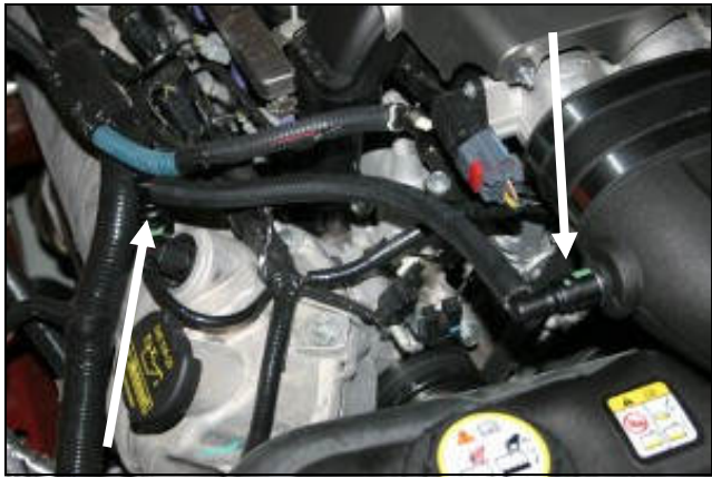
16. Install the two factory connectors from step #15 into each end of the supplied 3/8"x12" breather hose (#9). Now reattach one connector to the valve cover, and the other end to the aluminum fitting on the intake tube.
