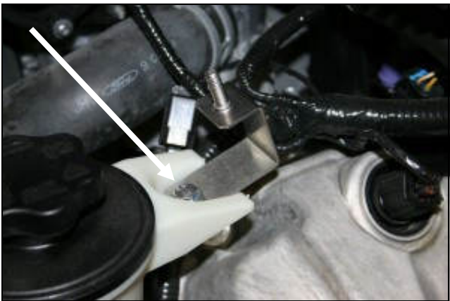
11. Install the bracket assembly from step #10 as shown. This bracket and 6mm bolt will secure the power steering reservoir and replaces the stud removed in step #9.
