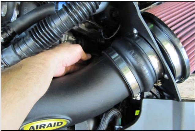
13. Reconnect the Mass Air Flow sensor, which is now located in the lower back side of the intake. Slide the locking tab back into the connector.
