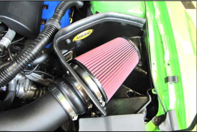
14. Install the Weather Strip onto the Cool Air Box with the contoured edge rolling away from the filter. Start at the front of the vehicle and work your way back.
