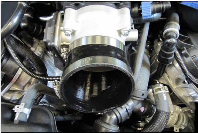
10. Install the Silicone Reducer (#6) and Hose clamps onto the throttle body. Place the #56 clamp (#15) on the Throttle body side of the reducer, and the #64 clamp (#14) on to the tube side.
