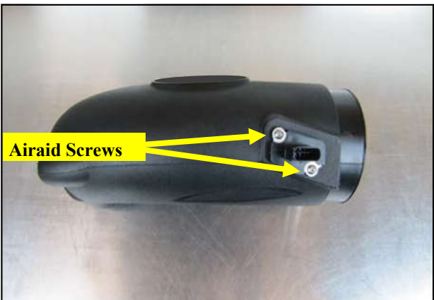
15. Transfer the Mass Airflow sensor into the Airaid Intake Tube as shown and secure it using the #8 Button Head Screws. Do Not Use the OEM hardware.
