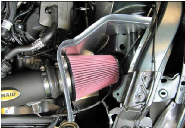
21. Install the Airaid Premium Filter onto the Filter Adapter. Install the weatherstrip on top of the Panel assembly as shown with the contour rolling away from the filter.
