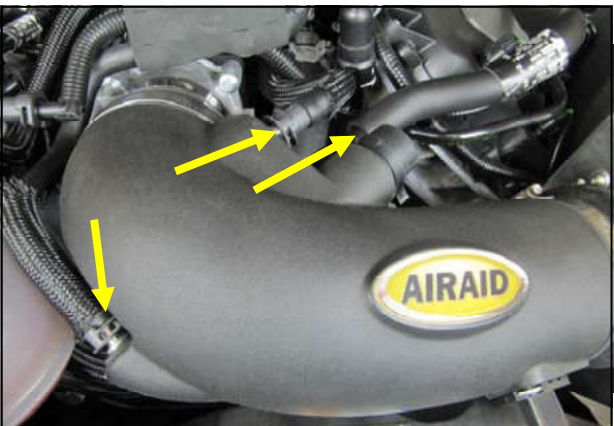
19. Insert the Intake Tube into the Hump Hose and Reducer then tighten all 4 Intake Clamps. Reconnect the factory breather lines. Apply the Airaid Bubble Decal onto the Intake Tube as shown.
