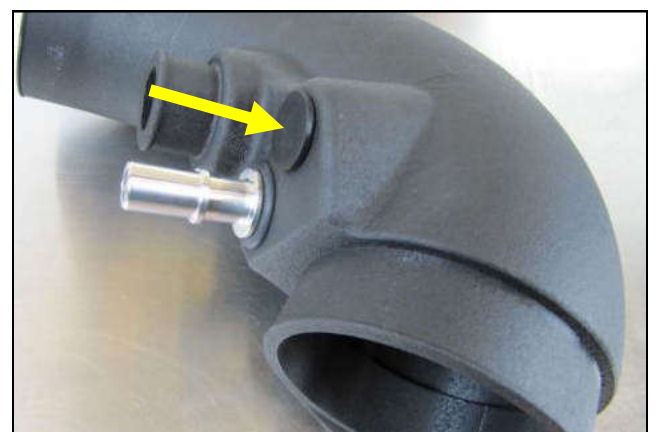
6. Manual transmission vehicles will not need the 3/8" components and will use the Blind Grommet.
