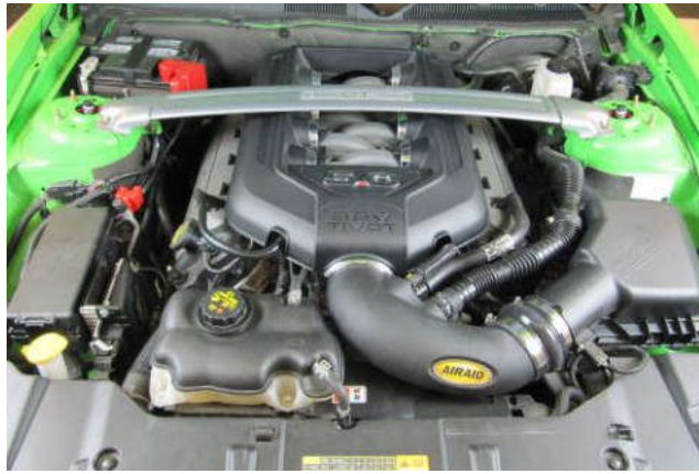
11. Reinstall the engine cover and Reinstall the strut tower brace, if so equipped. Reconnect the Battery terminal.
