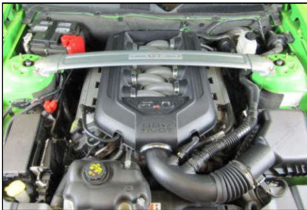
1. Disconnect the negative battery terminal. Remove the strut tower brace, if so equipped.
