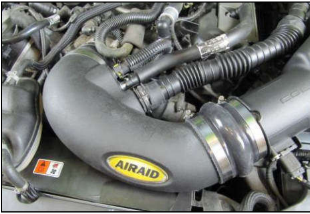
10. Connect the breather lines from step 3. to the Airaid intake Tube.
