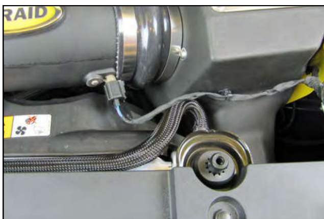
20. Reconnect the air temp sensor and plug the wire harness anchor into the Airbox.
