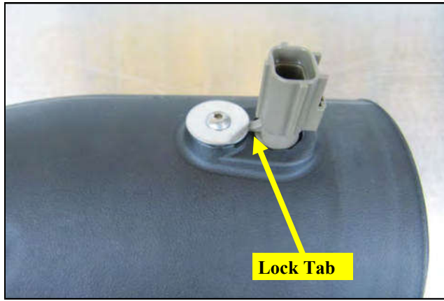
11. Insert the air temperature sensor into the Airaid intake tube as shown and secure it using the #8 Screw and Washer.
