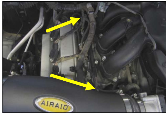
12. replace the OEM vacuum line on the fuel pressure regulator with the supplied 20 1/2" 1/8" line. Connect the 1/8" line to the small Fitting on the Intake tube.
