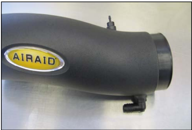
9. Install the 1/8" and 3/8" barbed fittings (#s 11 and 12) into the Airaid Intake Tube. Apply the Airaid Bubble Decal onto the Intake Tube as shown.
