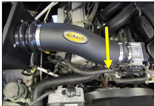
13. Connect the factory crank case breather line to the 3/8 Barbed Elbow on the Intake Tube.
