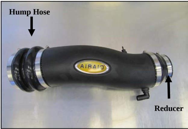
10. Slide the Hump Hose (#6), and two #68 Hose Clamps (#21), onto the Intake Tube as shown. Slide the Reducing Coupler (#7) and the #48 (#19) and #64 Clamps (#20) on the other end of the Intake Tube. Leave the Clamps loose for now.
