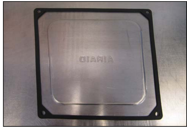
15. Place the Gasket (#8) onto the underside of the Air Box Lid (#4) and peel off the protective film. Mount the lid on the Air Box using four 1/4-20 x 1/2" Button Head Bolts (#16), and 1/4" Flat washers (#17).
