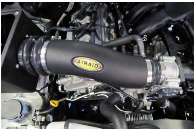
11. Install the Airaid intake tube onto the cold air box and the throttle body, align and tighten all four of the Clamps. Reconnect the mass air flow sensor.
