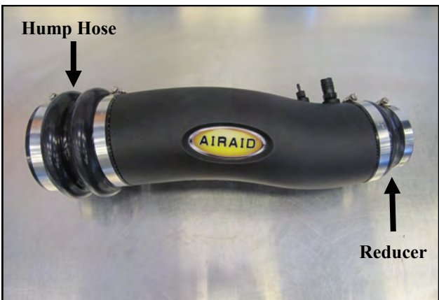
10. Slide the hump hose, and two #72 hose clamps onto the intake tube as shown. Slide the reducing coupler and the #48 and #64 clamps on the other end of the intake tube. Leave the clamps loose for now.
