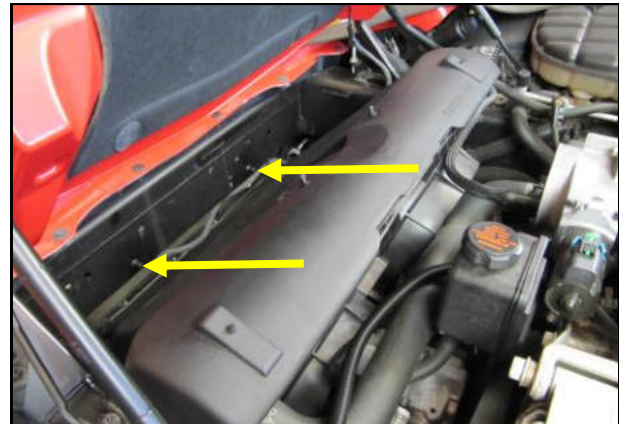
6. Inspect the inner bumper area and verify that none of the air box mounting grommets were retained during disassembly.
