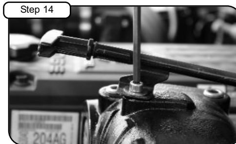
Step 14 Install the engine oil dipstick using M6 fender washer and socket cap screw provided. Tighten using 5mm allen key (See notes 1, 2 & 3). Attach the engine wire harness to the aFe manifold.
