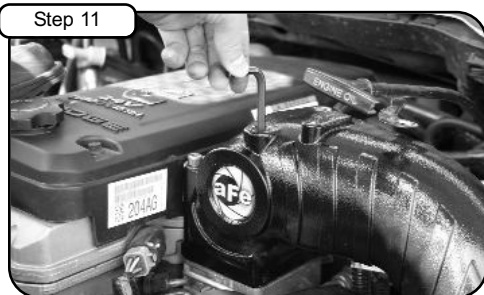
Step 11 With 6mm hexagonal bit provided and 6mm socket, install the four mounting bolts. Do not tighten completely!
