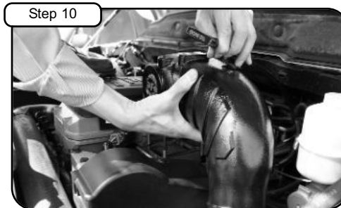
Step 10 Carefully install aFe manifold into vehicle. Guide bolts through gaskets and air grid heater. Insert aFe manifold into intercooler coupler hose.
