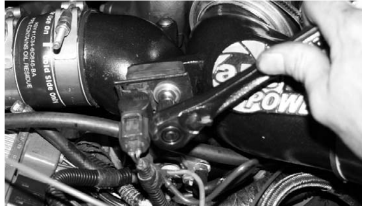
31- Now reinstall the boost control module. Reconnect battery.
