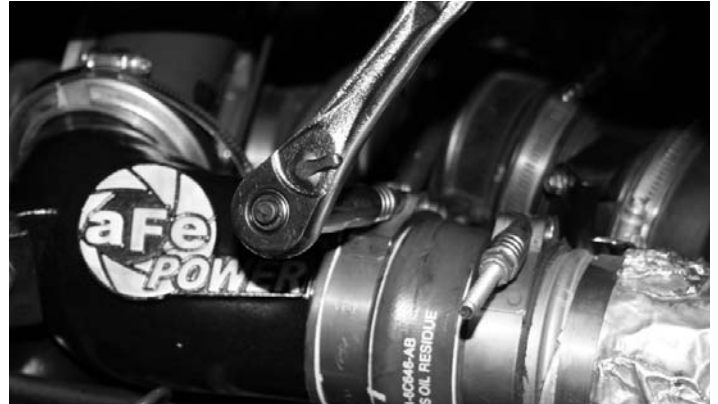
30- Install the hot side intercooler tube coupling onto the turbo manifold. Torque clamp to 9 Ft. Lbs.
