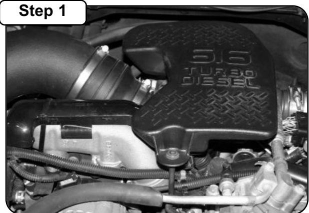
Stock turbo inlet tube.
