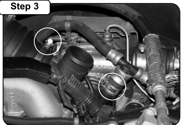
Open clamp on CCV hose coupler with pliers and remove coupler from the stock turbo inlet tube. Loosen air intake coupler clamp at stock turbo inlet tube with flathead screw driver or 5/16" socket driver.
