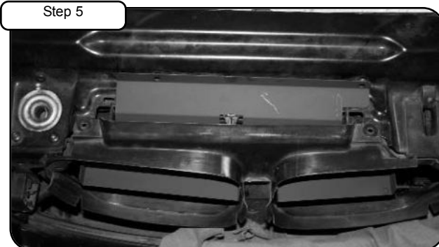
Grill support should pass through the clearance hole in the DAS.
