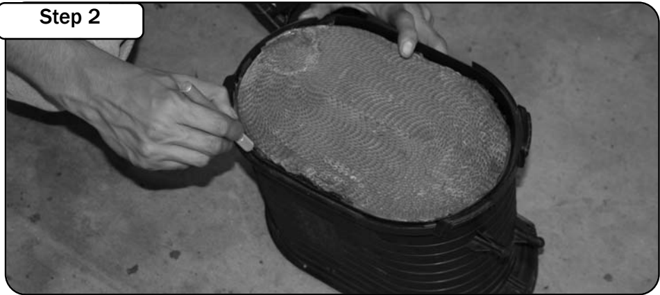
With a knife or sharp blade carefully cut along the edge of the OE air filter from the side opposite seal. Discard the air filter internals.
