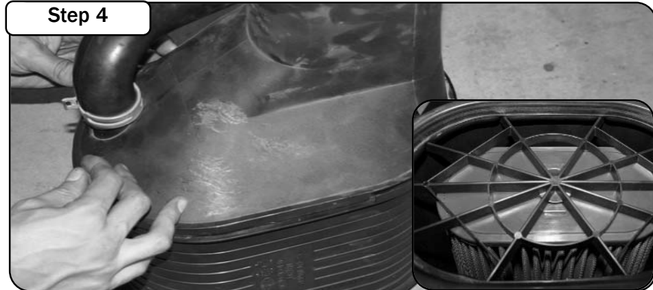
Re-assemble the air filter assembly. Verify engagement grooves are positioned as shown to ensure correct installation. Reinstall assembly back into engine.
