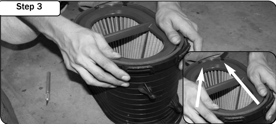
Carefully slide the air filter into the canister as shown above. Pay close attention to the alignment of the mounting slots relative to the filter housing.
