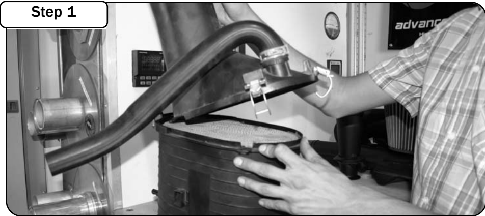
Remove the intake system which includes the air filter. Separate the air filter from the intake system.
