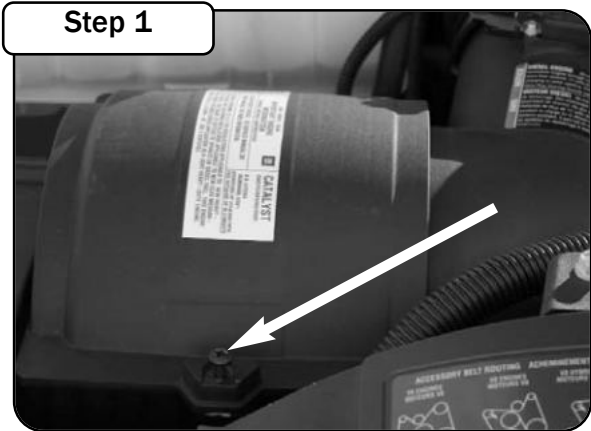
Step 1 Loosen the phillips screw on the air box and remove the cover to access the air filter.
