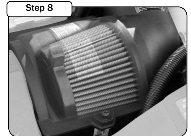
Step 8 Screw the air filter cover down. Verify the air box cover closes correctly. Your installation is now complete.
