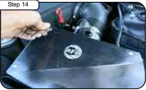
Install cover using button head screws provided and tighten using 5/32" allen key. Re-connect MAF sensor harness.
