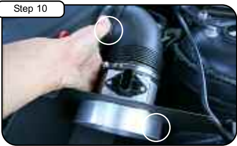
Loosen clamp on plenum box and position to new adaptor. Do not tighten.
