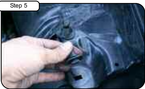
Turn and remove air box clips out of vehicle.
