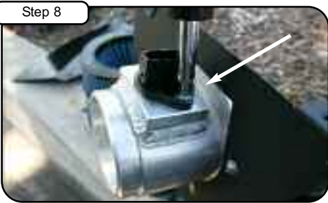
Install MAF sensor to filter adaptor using the 2 M4 screws provided and tighten using flat head screwdriver.
