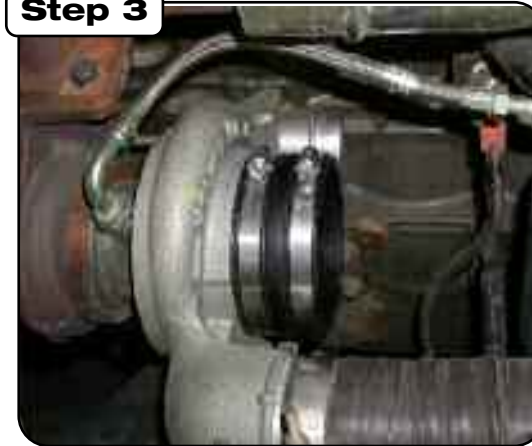
With both clamps on elbow coupler, place shorter (4" x 2-1/2") hi temp coupler on turbo inlet.
