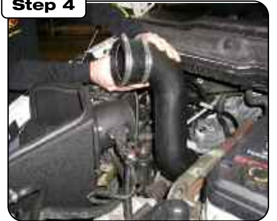
With longer (4" x 3") coupler slid onto the longer end of 419 tube, position the tube into place in the coupler on the turbo inlet. Then line up the top of tube and filter tube so you can slip the straight coupler over both tubes.
