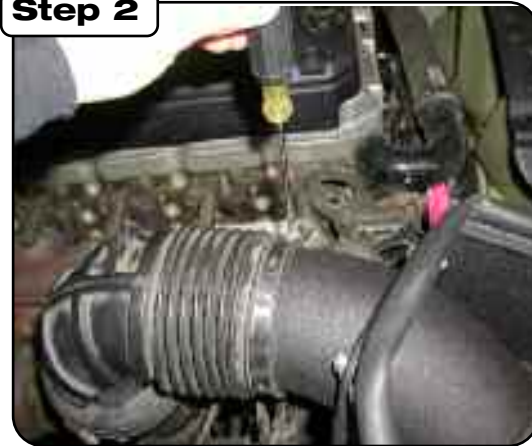
Loosen clamp for stock intake tube at turbo inlet and also loosen clamp at filter tube. Remove stock intake tube.
