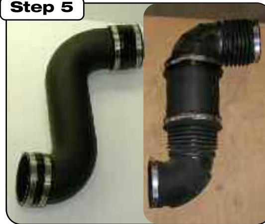
Compare the difference between stock and the Torque Booster Tube. Re-check clamps and connections and retighten after a few hours of operation.
