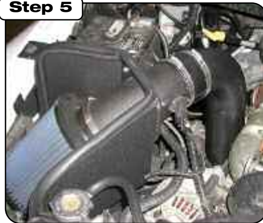
Once all pieces are set into place go through and tighten up all clamps.
