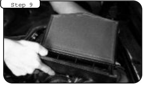
Step 9 Open the air filter access tray on the side of the air box and remove the OE air filter.
