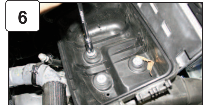
With 10mm socket or wrench, carefully remove bottom air box assembly out of vehicle. Pull back harness on back of air box.
