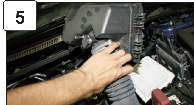
Remove upper half of air box and stock tube assembly.
