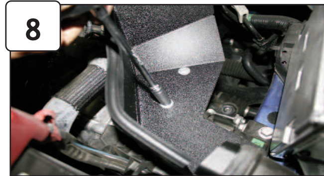
Install housing into vehicle and position. Secure housing using provided M6 screws and flat washers. Tighten using 10mm socket or wrench.
