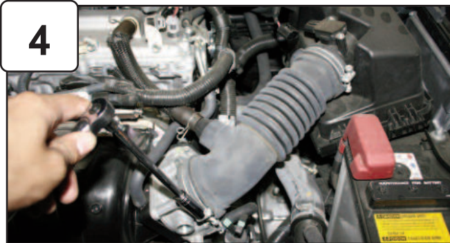
With 10mm socket or wrench loosen clamp on throttle body. Disconnect MAF sensor harness. Remove crank case line.
